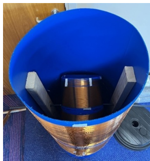
Variometer – rotating inner barrel for inductance adjustment
